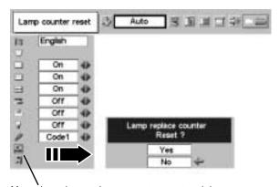
Move the pointer to Lamp counter reset and then press SET button. The message "Lamp replace counter reset?" is displayed.
